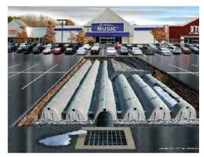
Figure B.11—Rendering of subsurface infiltration structure.
