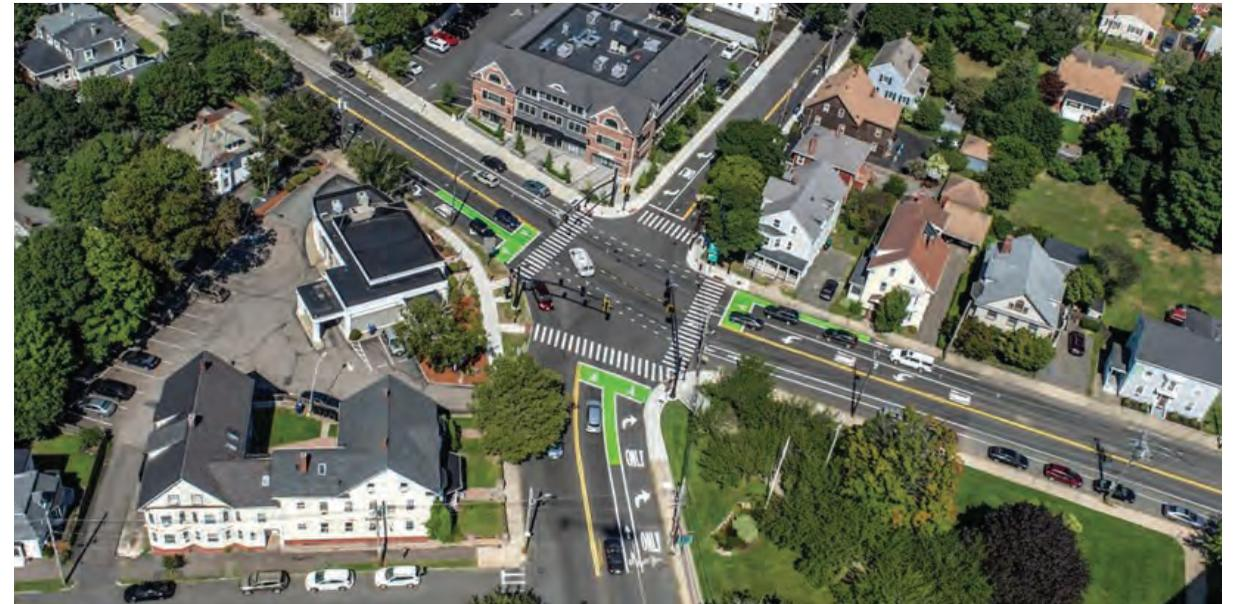
Figure 10-9. Rantoul Street in Beverly was successfully dieted for most of its length with a variety of tools, including new on-street parking, bike lanes and removal of excess lanes.
