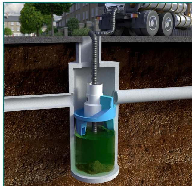
Fig 3. Maintenance is done with a vector truck
