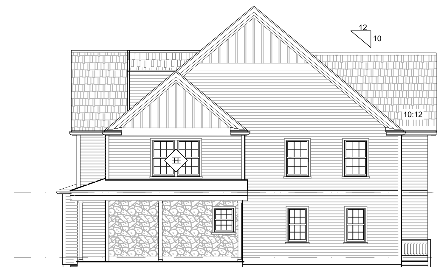
2 SOUTH ELEVATION (PAGE STREET) SCALE: 1/8" = 1'-0"
